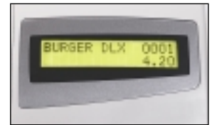
The 2-line alphanumeric backlit LCD display shows the item and price to minimize operator errors.
